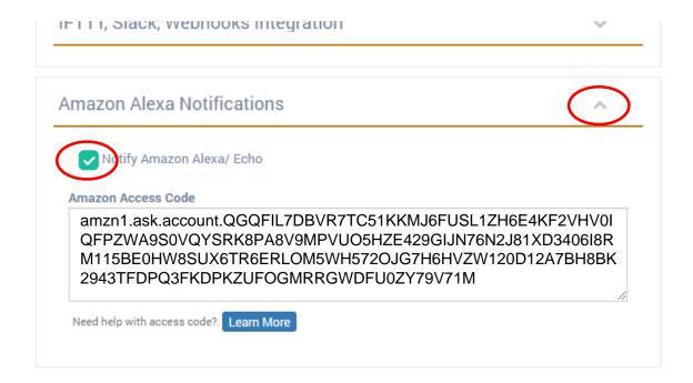
**G.** Scroll Down to the bottom, and click "Save Settings" button. That is it. Now, you can trigger your sensor to test the notifications. When the sensor goes to alarm, the message will be pushed to your alexa device.
